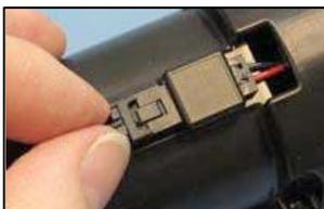
The battery is connected to VR2W on the side of the case. When installing the battery, listen for a "click" and watch that light flashes four times and then twice quickly every 5 seconds. When disconnecting battery, press the release tab on the battery connector and then pull connector halves apart.
